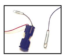
3. Tape your paper clips onto a piece of cardboard, so the small loop of both paperclips is on the bottom of the cardboard. Make sure they don't touch.
